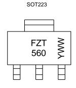
FZT 560 = Product Type Marking Code YWW = Date Code Marking Y or  $\overline{Y}$  = Last Digit of Year (ex: 5= 2015) WW or  $\overline{W}W$  = Week Code (01~53)
