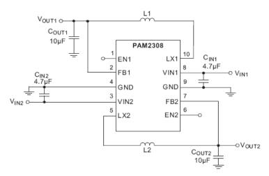
V<sub>OUTx</sub> = 1.2V, 1.5V, 1.8V, 2.5V, 2.8V or 3.3V Figure 2. Fixed Voltage Regulator
