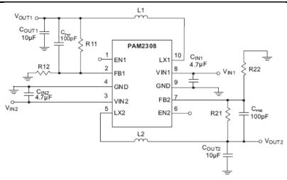
$$V_{OUTx} = V_{REF} \left( 1 + \frac{Rx1}{Rx2} \right)$$
