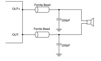
Figure 1: Ferrite Bead Filter to Reduce EMI
