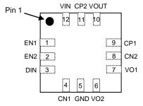
U-QFN3030-12 (Type A)/W-QFN2020-12 (Type US)
