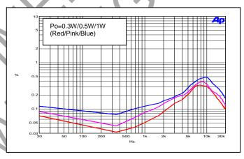
PSRR Vs. Frequency(RL=8Ω)
