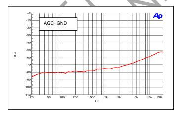
PSRR Vs. Frequency(RL= $4\Omega$ )
