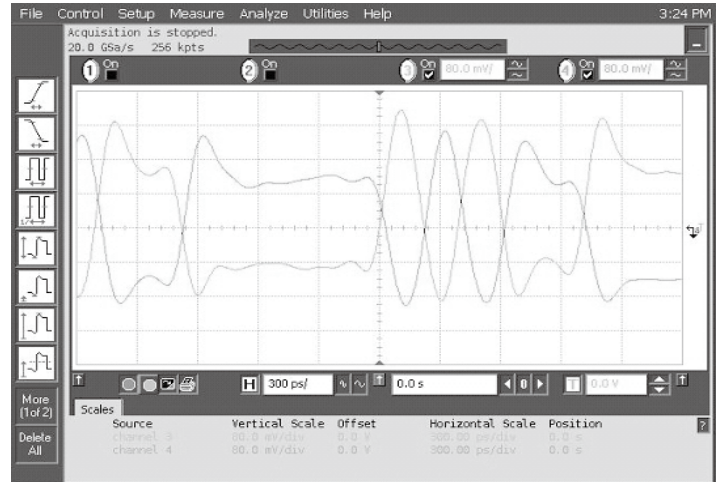
Data Waveforms, 2.5Gbps (left) & 5.0Gbps (right)
