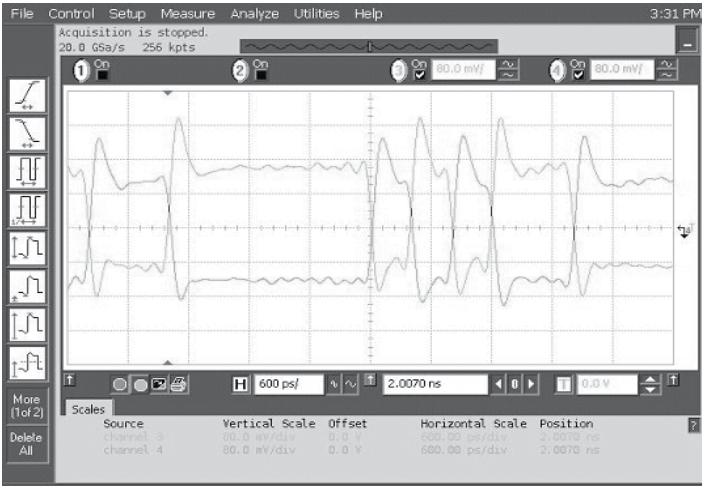
Data Waveforms, 2.5Gbps (left) & 5.0Gbps (right)
