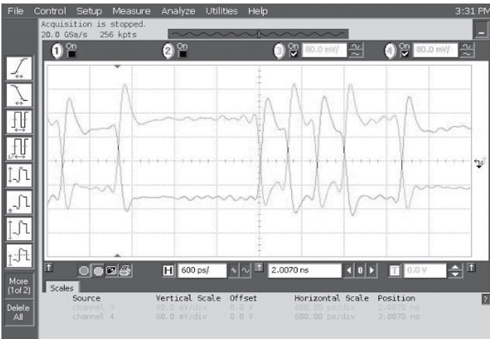
Data Waveforms, 3.0Gbps (left) & 6.0Gbps (right)
