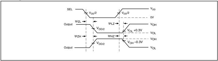
**Voltage Waveforms Enable and Disable Times**
