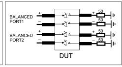
Diff. Insertion Loss and Return Test Circuit
