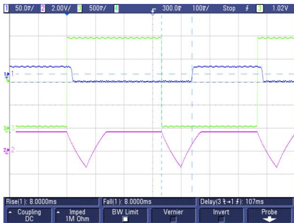
Figure 10, Soft-start with C_{SSCAP} = 10nF , V_{NC} = +50mV , V_{NO} = 0V Channel 1 = COM Channel 2 = SSCAP Channel 3 = IN
