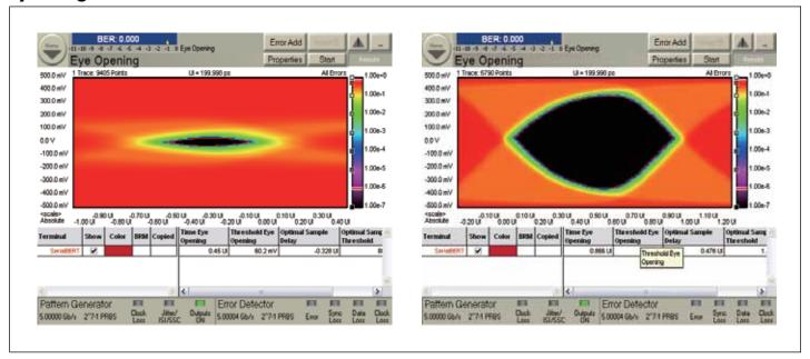
Left: Input Eye Diagram, Left: Output Eye Diagram, Trace length: 36-inch, 5.0 Gb/s
