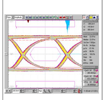
Fig. 2. Output Eye Opening at 3.3Gbp, 500mV swing and double termination, 0dB pre-emphasis, 48" input Trace, 9dB EQ setting
