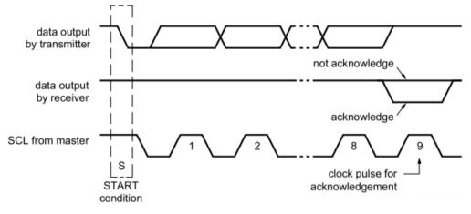
Figure 10. Acknowledgment on I2C Bus
