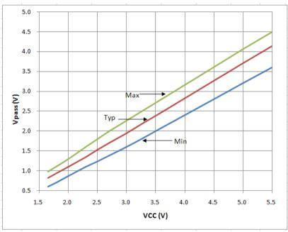
Figure 6:Vpass voltage VS Vcc
