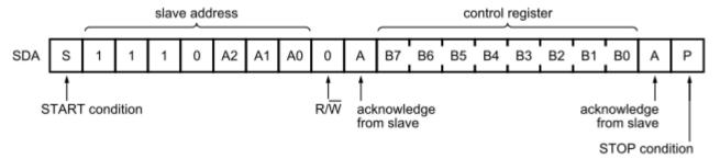
Figure 11. Write Control Register
