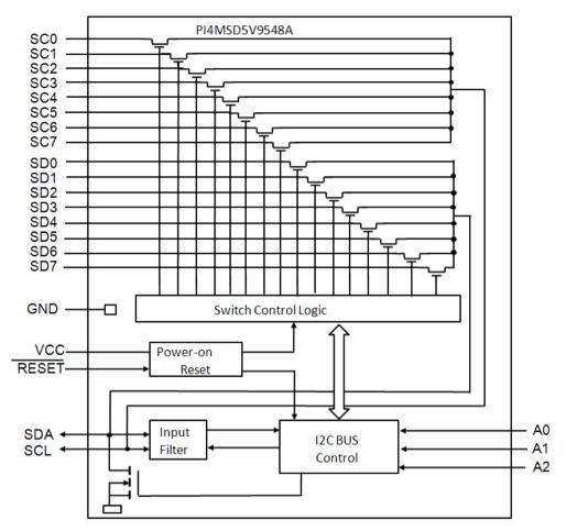
Figure 1: Block Diagram
