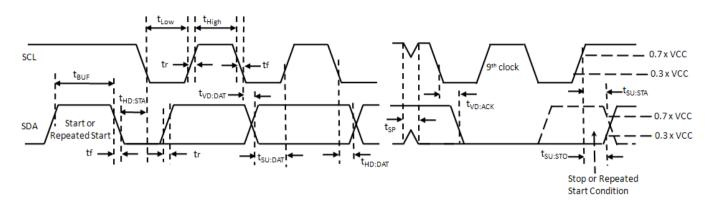
Figure 2. Definition of timing on the I2C-bus
