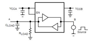
Figure 3. Driving B Test Circuit
