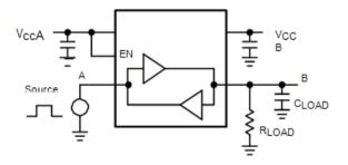
Figure 2. Driving A Test Circuit
