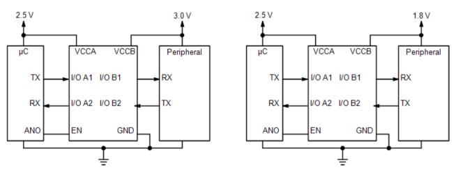
Figure 9 Application Example for A > B
