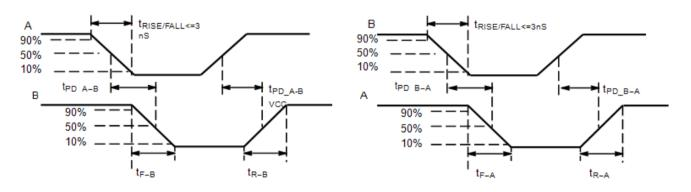
Figure 4. Definition of Timing Specification Parameters
