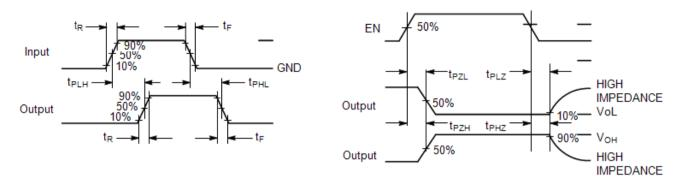
Figure 5. Timing Definitions for Propagation Delays and Enable/Disable Measurement
