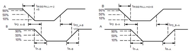
Figure 3. Definition of Timing Specification Parameters
