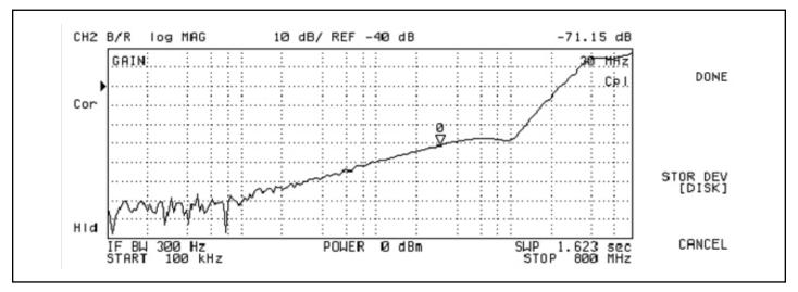
Figure 2. Off Isolation vs Frequency
