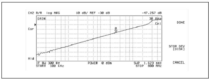
Figure 3. Crosstalk vs Frequency
