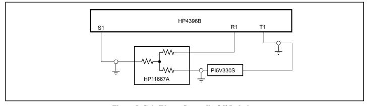
Figure 5. Gain/Phase, Crosstalk, Off-Isolation
