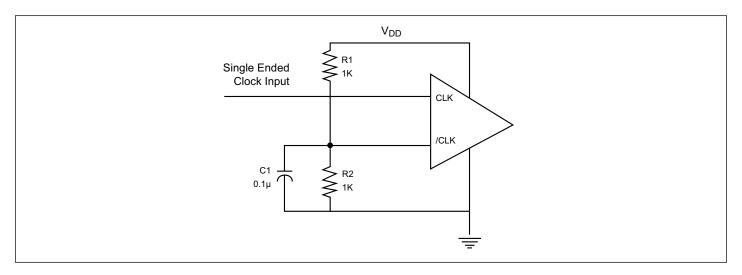
Figure 1. Single-ended Input to Differential Input Device
