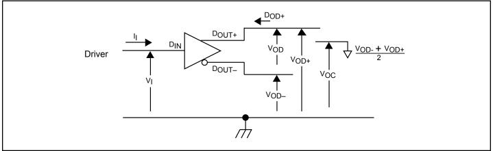
Figure 1. Driver Voltage and Current Definitions
