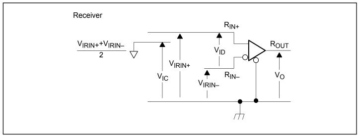
**Figure 4. Receiver Voltage Definitions**
