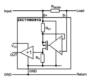
Fig. 20 Typical Configuration of ZXCT1080Q/81Q
