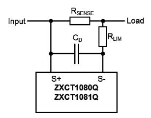
Fig. 21 Protection/Error Sources for ZXCT1080
