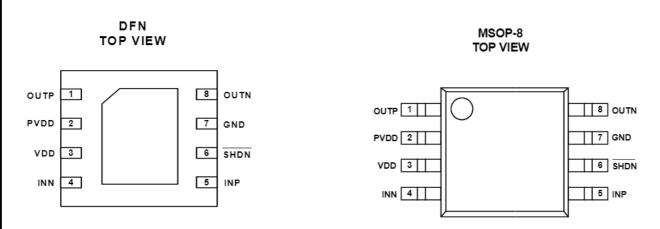
Figure 1 Pin Assignment (Top View)
