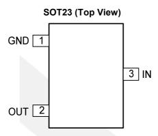
Figure 1 Pin Assignment
