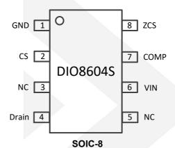
Figure 2 Pin Assignment (Top View)
