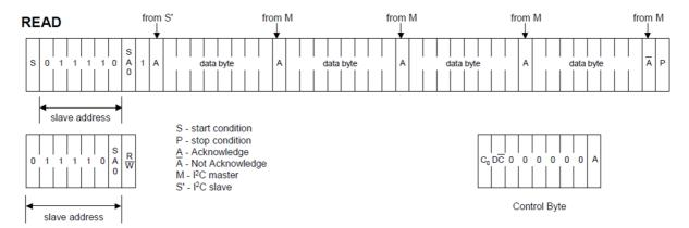
(a)I2C address bit (SA0) The slave address is following the start condition for recognition use. Two 7-bit slave addresses are "b0111100" or "b0111101" by changing the SA0 to LOW or HIGH (A0 pin acts as SA0).
