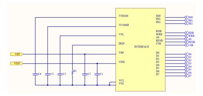
Recommended Components : C1: 0.1uF C2,C3,C4,C5: 4.7µF R1: about 750kOhm , R1 = (Voltage at IREF – GND)/IREF
