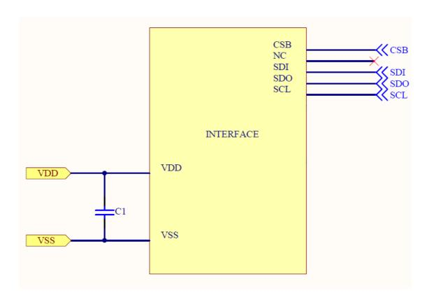
Pin connected to MCU interface: CSB,SDI,SDO,SCL
