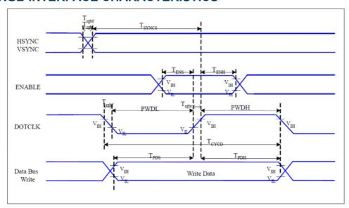
Figure 6 RGB Interface Timing Characteristics
