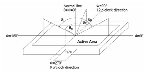
FIG. 3 The definition of Viewing Angle
