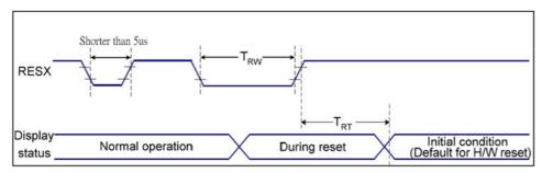
Figure 7 Reset Timing
