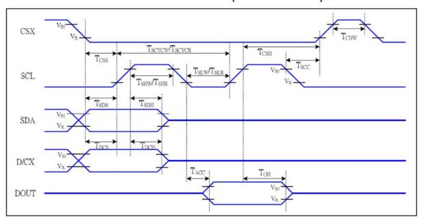
Figure 5 4-line serial Interface Timing Characteristics
