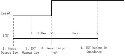
Fig.8(b) Timing of setting slave address
