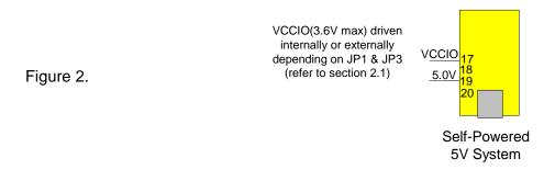
Figure 2 illustrates a typical USB self-powered configuration. A USB self-powered device gets its power from its own power supply and does not draw current from the USB bus.
