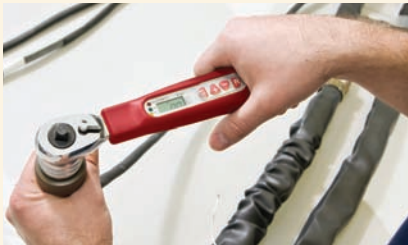
Digital torque wrench, adaptor, connector, strain relief
