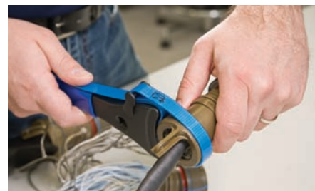
Strap wrench, strain relief, connector
