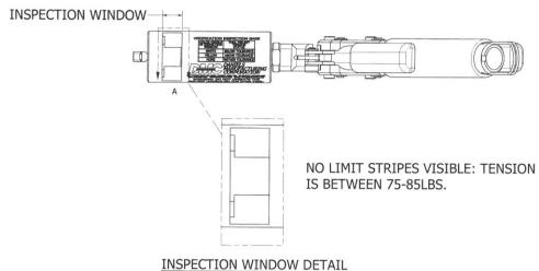
If any amount of the yellow stripe is visible, the tension applied to the band by the DBS-2200 is above 85LBS. This indicates that the tension setting for the DBS-2200 must be adjusted. (See section 3.2 for adjustment instructions.)
