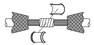
If the shield has been cut and separated to expose the wires requiring service and the required service has been completed, the wire bundle is then protected by a few wraps of self-vulcanizing tape followed by 2–3 layers of teflon tape. An appropriate size split-ring set is then selected and installed. One layer of teflon tape is applied over the split ring set to hold the halves in position while the next steps are being performed.
