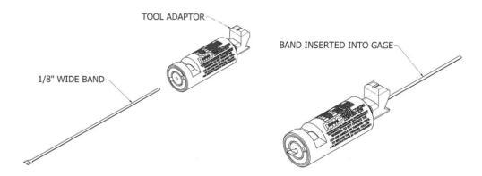
Step 2: Insert the end of the band into the DBS-2200
