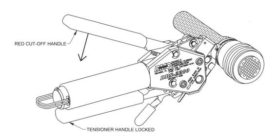
Step 6: Remove excess band material
