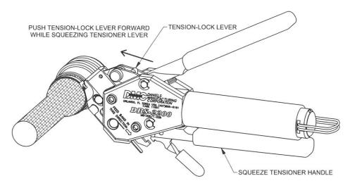
To loosen or remove the looped band after locking the tensioner handle at the precalibrated tension, squeeze the tensioner handle and push the tension-lock lever forward. While holding the tension-lock lever forward, release the tensioner handle. The tensioner handle will open fully. Squeeze the release lever and pull the looped band away from the nose of the tool.
