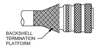
The braid is pushed into position over the backshell termination platform. Care must be taken to make sure the weave is uniform and no large "windows" are present. A shield termination band is loaded into the tool. If the band is uncurled it must be double looped through the buckle before termination. The band is then slid into a position of alignment with the backshell termination platform.
