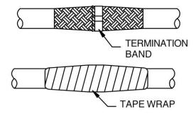
Heat-shrinkable tape is then applied over the splice. When a jacketed cable is used, be sure the tape extends onto the jacket in both directions.
