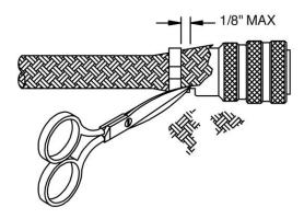
For braiding a non-jacket cable use fine point shears to trim the excess braid as close to the connector side of the bands as possible. Do not leave any unsecured braid wires longer than 1/8 inch. Do not allow the trimmed wires to fall in any areas where they may present a foreign object damage hazard. If a shrink boot or other covering is used, the excess braid may be folded back over the band.
