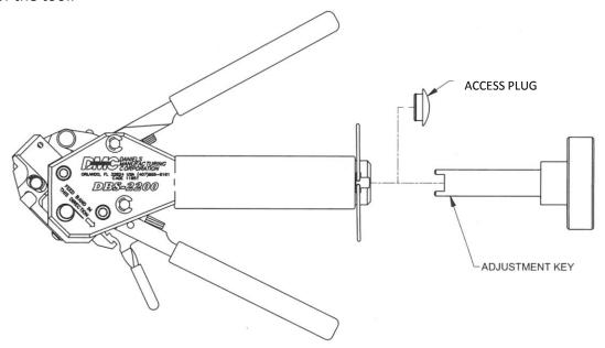
Step 2: Insert the adjustment key into the access hole
