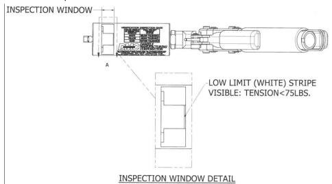
If no limit stripes are visible in the Inspection Window, the tension applied is between 75-85LBS. The Banding tool is within the acceptable range and does not require any adjustment.
