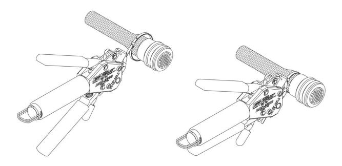
Apply an adequate amount of pressure in line with the cable as it enters the backshell to allow the 1/8 inch space to be reduced to zero. The tool is then activated to the preset tension, and terminated/cut using the procedure described in section 1.0 of this guide.
