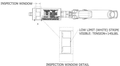
If no limit stripes are visible in the Inspection Window, the tension applied is between 145-155LBS. The Banding tool is within the acceptable range and does not require any adjustment.
