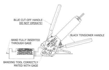
Align the tool's nose so that it butts up against the DBS-CG7 as shown below.
