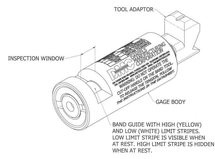
Warning: Keep the DBS-CG7 in a clean, dry place when not in use. Keep the inspection window free from dust and debris.
