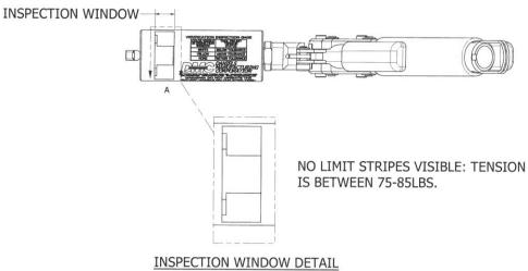
If any amount of the yellow stripe is visible, the tension applied to the band by the DBS-2200 is above 85LBS. This indicates that the tension setting for the DBS-2200 must be adjusted. (See section 1.2 for adjustment instructions.)
