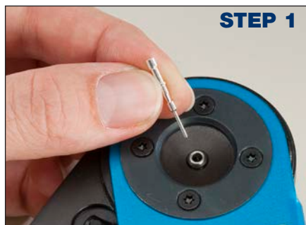
STEP 1 INSERT CONTACT
