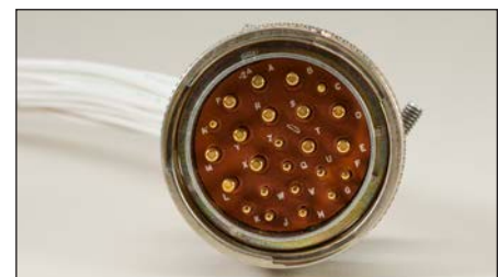
Connectors may contain several different size contacts.
