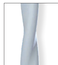
RIGHT HAND LAY "Z" DIRECTION
