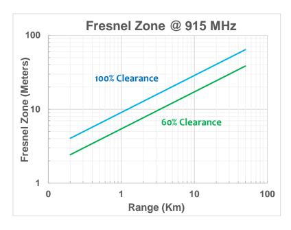
RF Line of Sight (LOS) is defined by <u>Fresnel Zones</u> which are ellipse shaped areas between any two radios. The radius of the Fresnel Zone at its widest point is shown the figure.
