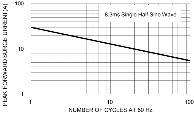
FIG. 3 MAXIMUM NON-REPETITIVE FORWARD SURGE CURRENT
