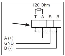
By short-circuiting pin B across pin T, the line can be terminated with a 120 Ohm resistance, already present inside the electronics.
