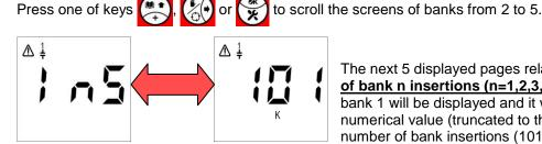
The next 5 displayed pages relate to the alarm **maximum number** of bank n insertions (n=1,2,3,4,5). At first the screen relating to bank 1 will be displayed and it will be alternately shown with the numerical value (truncated to the thousands) corresponding to the number of bank insertions (101000 in the example shown).
