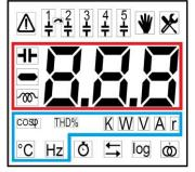
digits, the dot if necessary, the sign and the indication of the inductive or capacitive load, and the measuring unit and/or type of measurement (area highlighted in blue).
