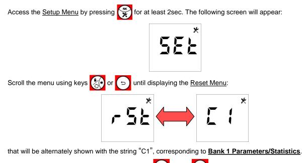
Access parameter editing mode by pressing key 🚑 or key 🥽, then use the same keys to scroll the values until reaching the desired parameter.
