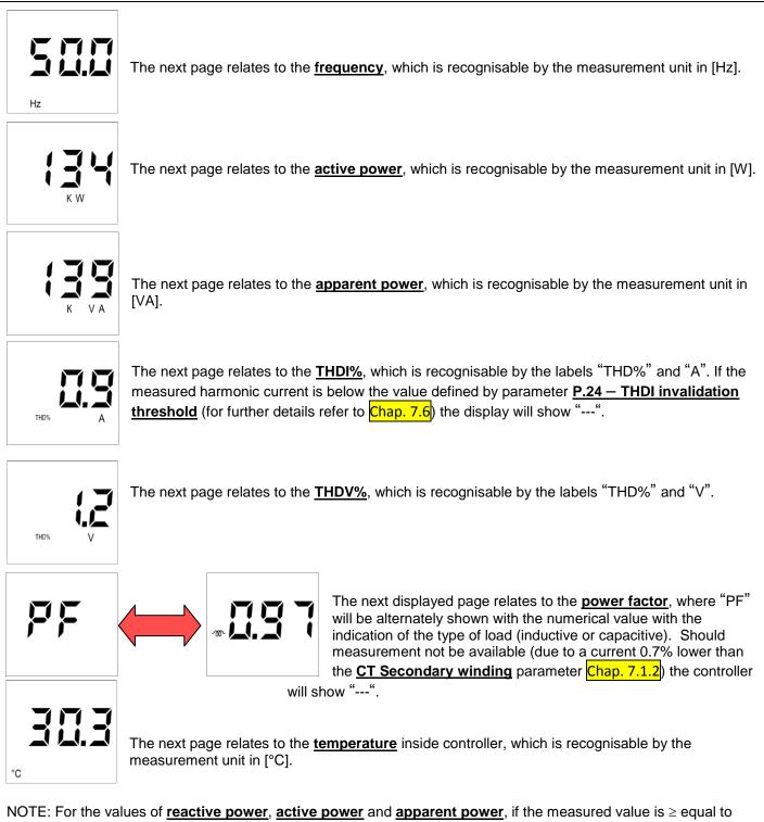
one MVAr, one MW and one MVA respectively, the following screen will be respectively displayed alternately with the numerical value.
