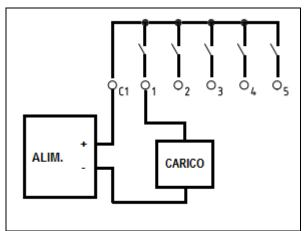
The contact is in NO (normally open) logic, and it closes if the output-associated alarm is activated.
