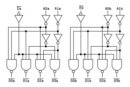
FIGURE 3. Logic diagram.
