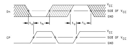
FIGURE 4. Switching waveforms and test circuit.
