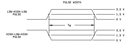
FIGURE 4. Switching waveforms and test circuit.
