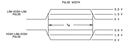
FIGURE 4. Switching waveforms and test circuit.
