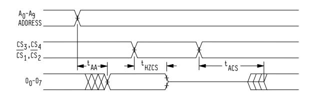
FIGURE 4. Switching waveforms.
