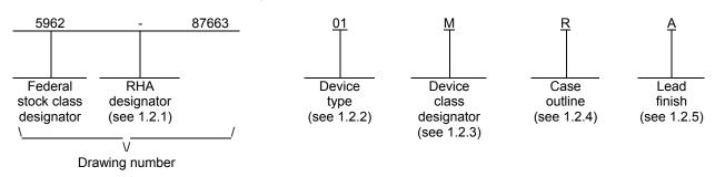
1.2.1 <u>RHA designator</u>. Device classes B, S, Q, and V RHA marked devices meet the MIL-PRF-38535 specified RHA levels and are marked with the appropriate RHA designator. Device class M RHA marked devices meet the MIL-PRF-38535, appendix A specified RHA levels and are marked with the appropriate RHA designator. A dash (-) indicates a non-RHA device.
