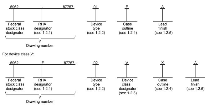
1.2.1 RHA designator. Device classes Q and V RHA marked devices meet the MIL-PRF-38535 specified RHA levels and are marked with the appropriate RHA designator. Device class M RHA marked devices meet the MIL-PRF-38535, appendix A specified RHA levels and are marked with the appropriate RHA designator. A dash (-) indicates a non-RHA device.
