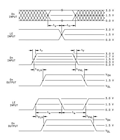
FIGURE 4. Switching waveforms and test circuit.
