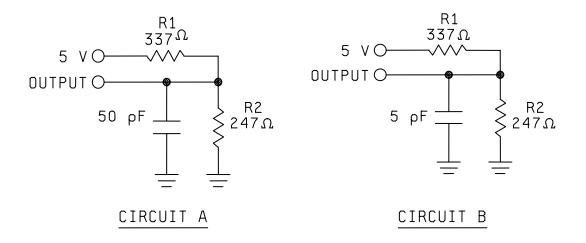
FIGURE 3. Output load circuit.
