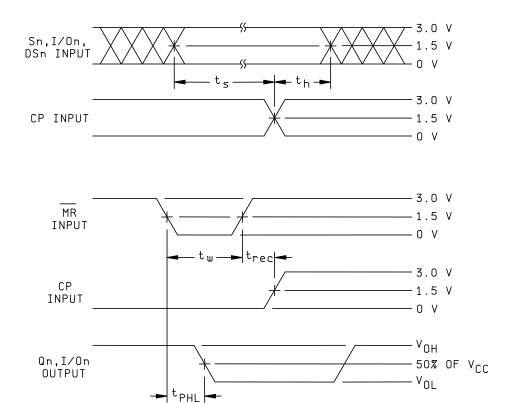
FIGURE 5. Switching waveforms and test circuit.
