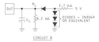
NOTE:  $C_L = 100 \text{ pF}$  including jig capacitance.
