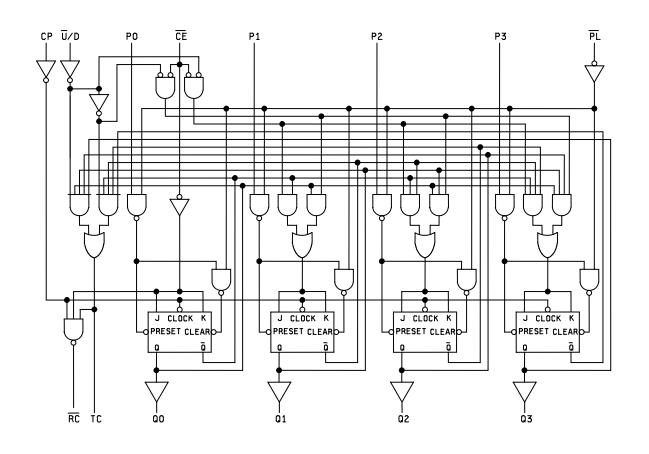
FIGURE 3. Logic diagram.
