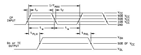
FIGURE 4. Switching waveforms and test circuit.
