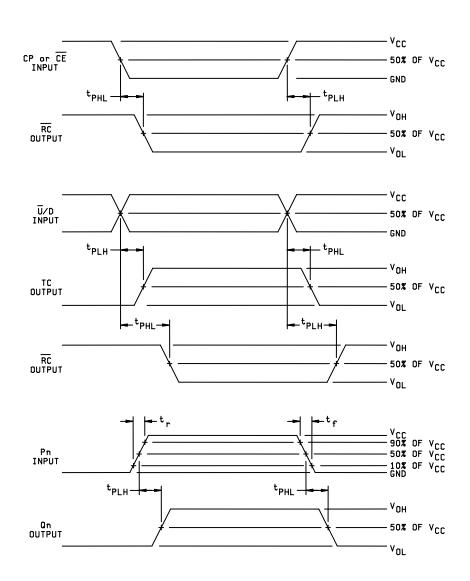
FIGURE 4. Switching waveforms and test circuit – Continued.
