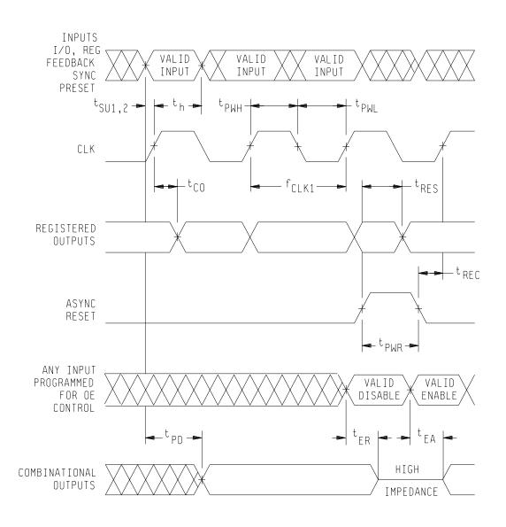
FIGURE 4. Switching waveforms.
