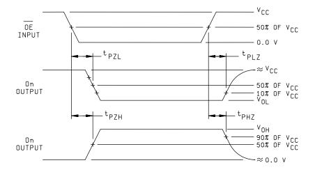
FIGURE 4. Switching waveforms and test circuit.
