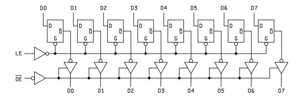
FIGURE 3. Logic diagram.
